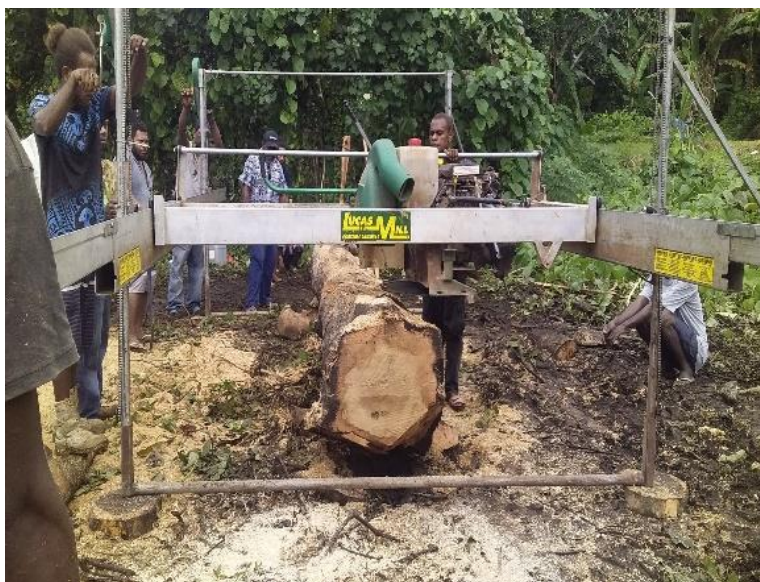
Figure 2. Practical skills session on setting up of log and sawmill for safe operation
